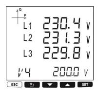
BUTTON NAME DISPLAYED MEASUREMENT SCREEN ESC (VIF) VOLTAGE (L-L)
